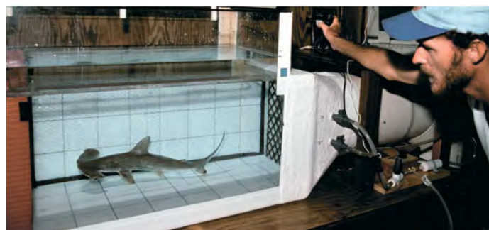
▲ Figure 40.18 Measuring the rate of oxygen consumption by a swimming shark. A researcher monitors the drop in oxygen level in the recirculating water of a juvenile hammerhead's tank.
