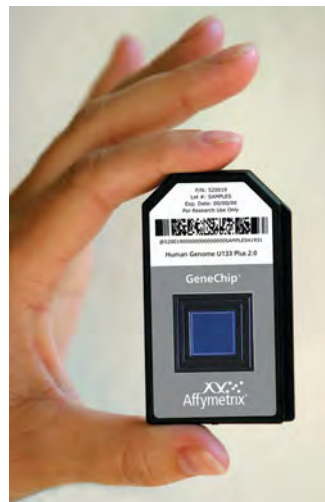
◀ Figure 21.6 A human gene microarray chip. Tiny spots of DNA arranged in a grid on this silicon wafer represent almost all of the genes in the human genome. Using this chip, researchers can analyze expression patterns for all these genes at the same time.
